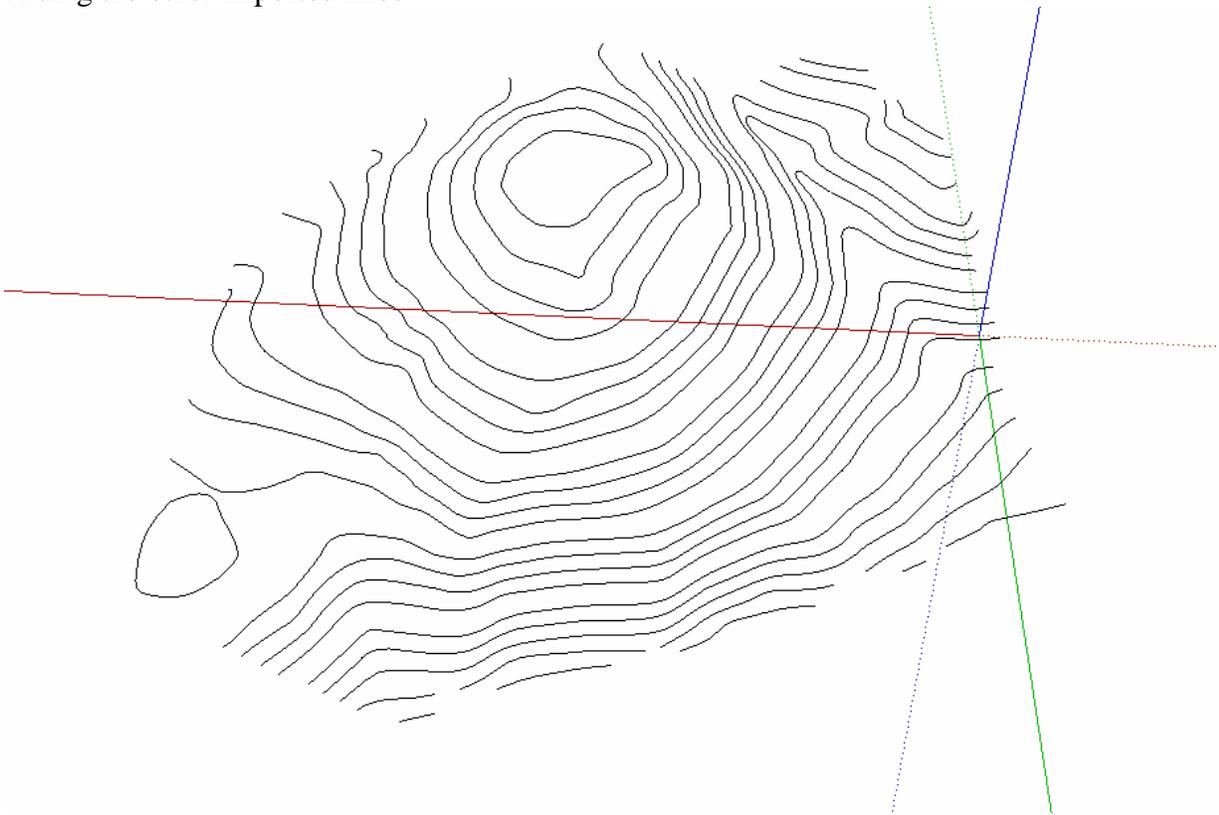
This time, I will select the whole contour and use this tool – The sand box tool. The first icon “from contours is the most important tool to generate the terrain.
